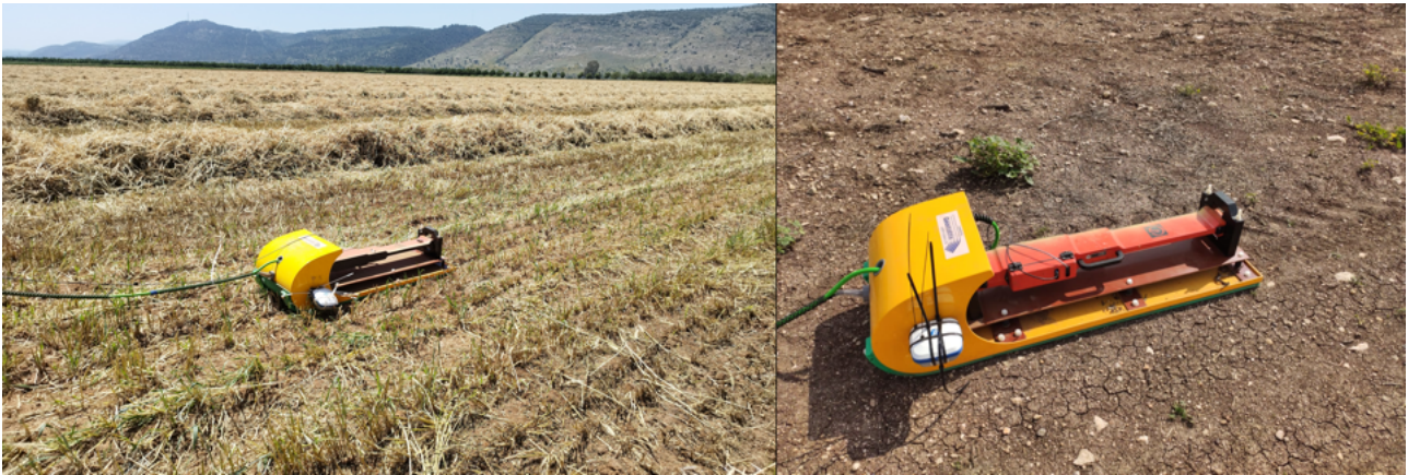
Figure 1: ECa survey equipment and study site. (a) Survey in progress in the Hula Valley study site, April 2023, showing wheat residue windrows and transect pattern. (b) EM38-MK2 electromagnetic induction sensor mounted on a nonconductive sled, sensor shown in horizontal dipole orientation.
