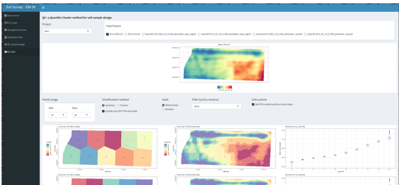
Figure 18: Screenshot of the shiny web application app-1, a tool for soil sampling design by ECa data, displaying a section of QC sample design results for n \in \{11 - 22\} sampling points.
