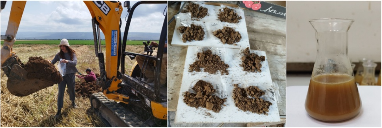
Figure 4: Soil sampling collection at the study site using a backhoe excavator (left); soil samples air-drying before PSD measurement (center); and soil sample pretreatment: a 1 g sample stirred with hydrogen peroxide solution for organic matter removal.
