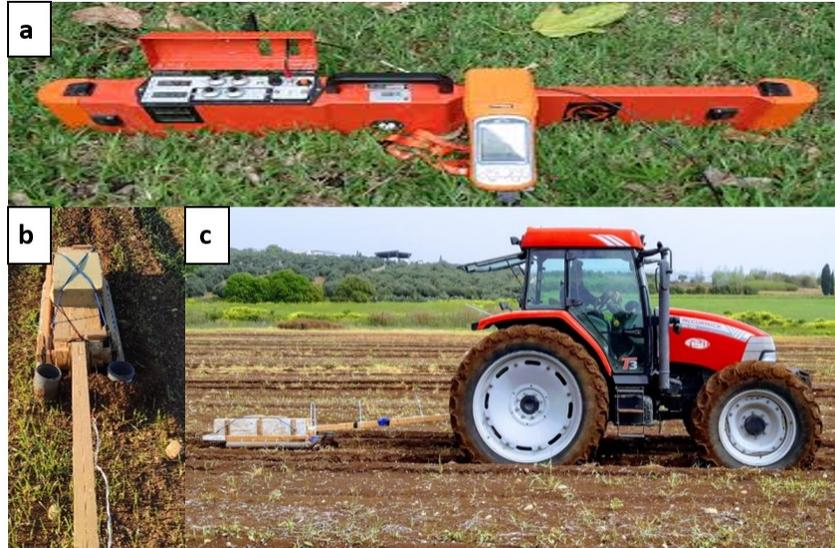
Figure 3.1: **a.** EM38-MK2 EMI device and Archer XF101 GPS device. **b.** Special wagon without metal parts for containing the EMI device. **c.** Vehicle dragging the special wagon with the EM38-MK device inside it.
